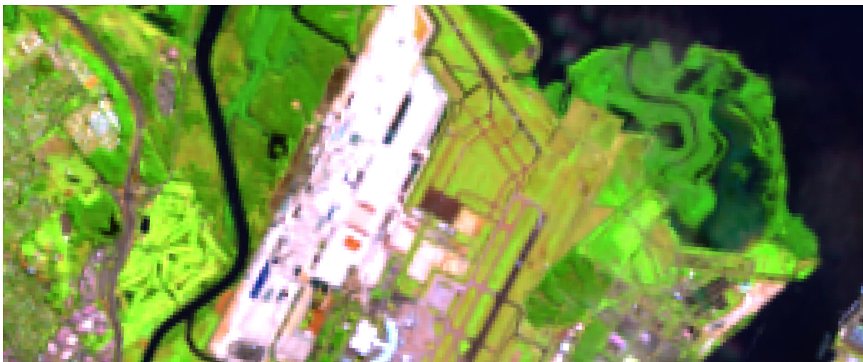
c. Nearest neighbouring resampling with picking and binning
